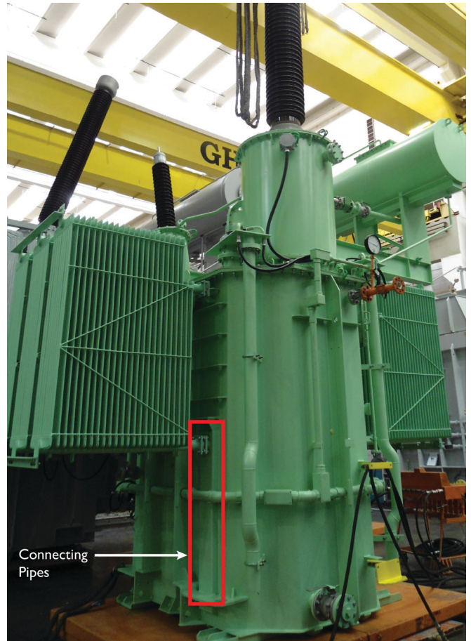
FIGURE 1. Shunt reactor. In the original design of the oil circuit the radiator is connected to the tank by pipes enclosed in rectangular boxes welded to the exterior of the reactor.
