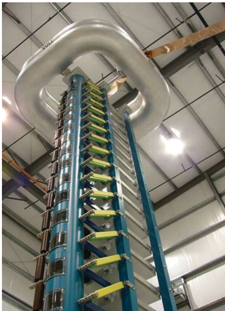
FIGURE 1. High-voltage generator (2.4 MV Marx generator) operated by NTS.
