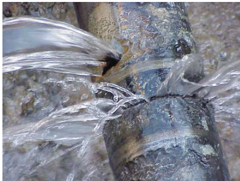
FIGURE 1. Left: Leaky pipe under investigation. Right: Schematic of leak detection setup. A leak is bracketed by two sensors whose distance is D . The leak sound propagates in both directions and a correlator measures the time it takes to reach each sensor. Based on the speed of sound in the pipes, the exact leak location can be found.
