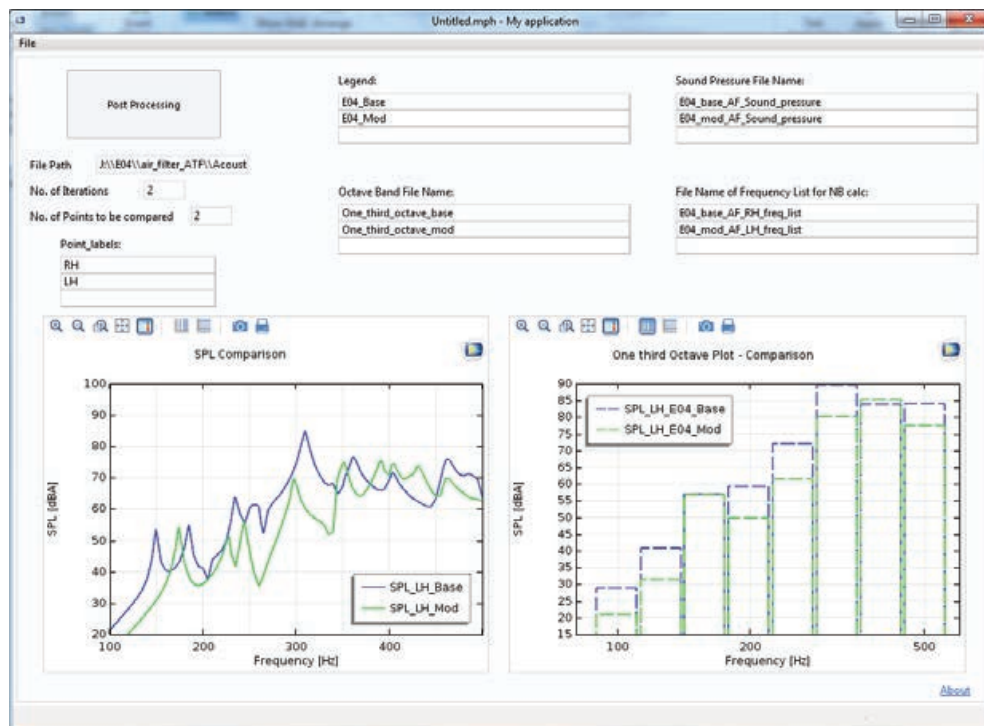
FIGURE 6. With the Application Builder, Mahindra engineers created an easy-to-use simulation app that is used to compare analysis files and plot sound pressure level (SPL) data.
